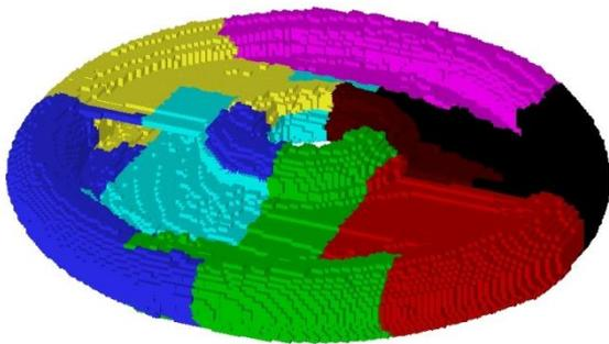
Sample domain decomposition using space filling curves
