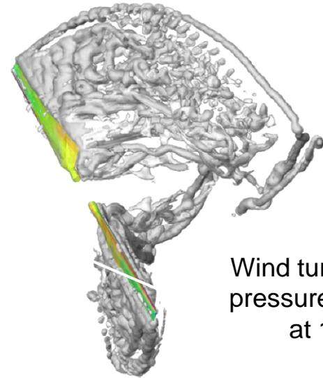
Wind turbine blade pressure and wake at 15m/s
