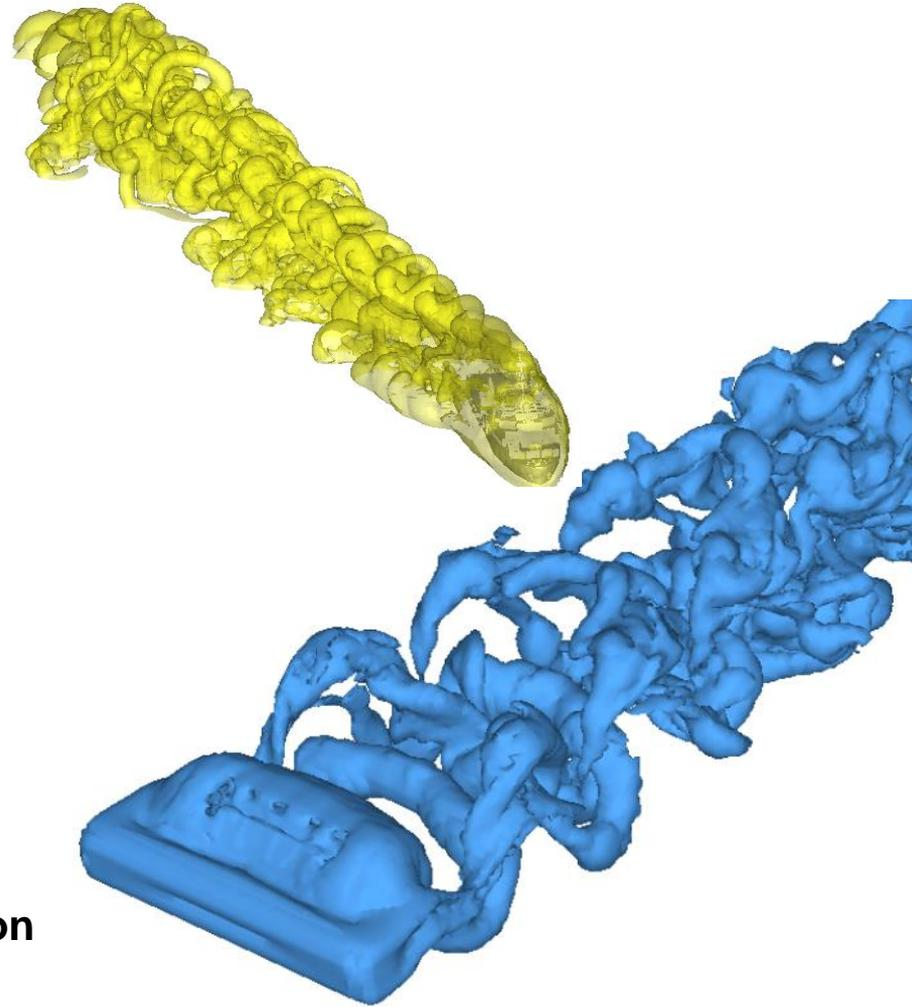
Hybrid overset prediction of a ship air wake and the wake behind a wing at 90° angle of attack
