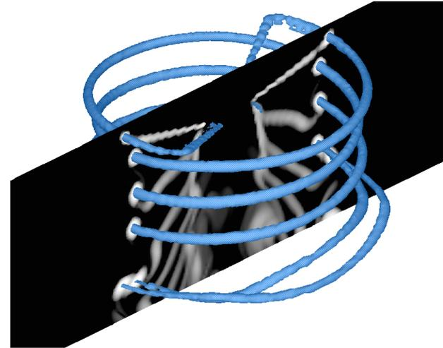
Grid-based prediction of hovering rotor wake
