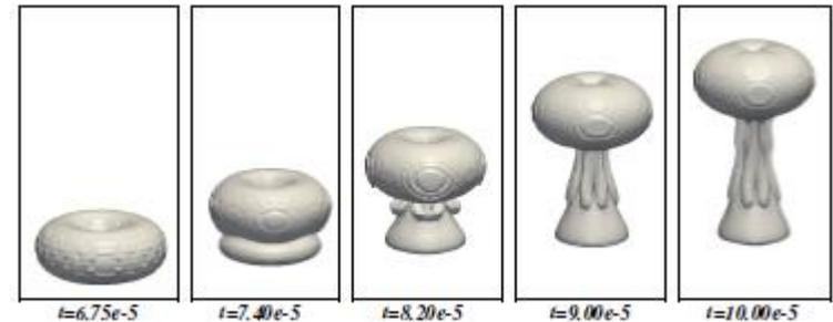
Grid-based prediction of viscous vortex ring evolution from Harris *et al* AIAA-2010-1072
