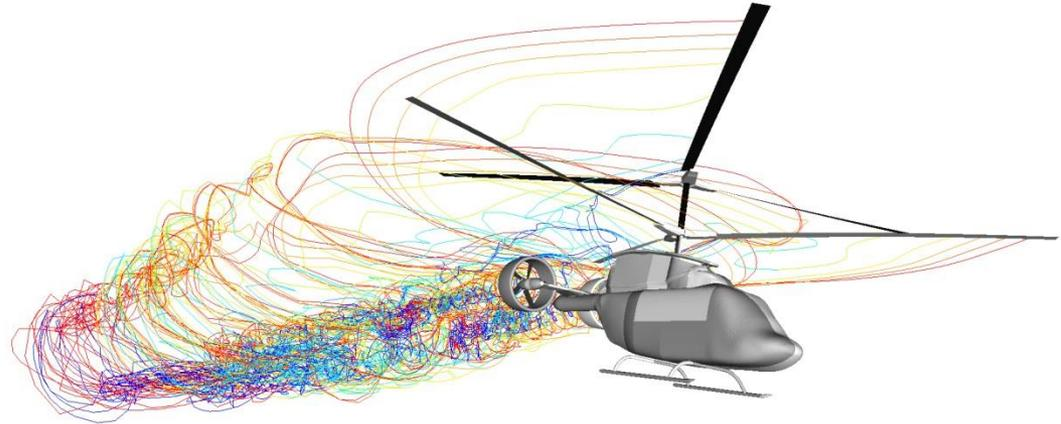
CHARM filament wake for an advanced coaxial compound
