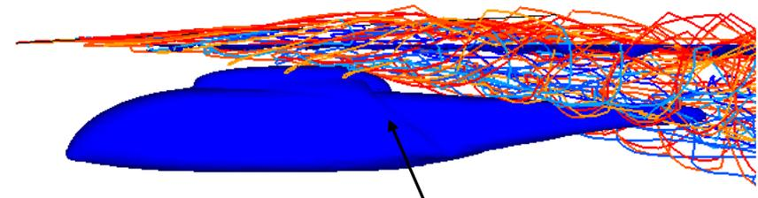
Flow separation on fuselage
