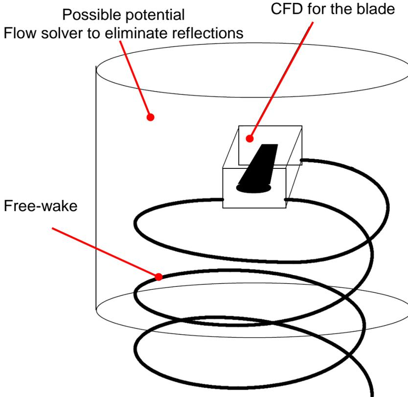
Schematic of idealized CFD/free-wake coupling
